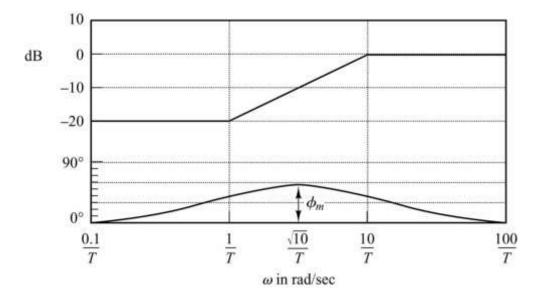
**Example** Lead design; Desired system is  $K_v$  of 20 sec<sup>-1</sup>, 15% overshoot related to PM of 53 degree (damping ratio of 0.516)
