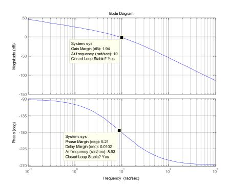
Phase margin(PM)= 5.2 deg. at 8.93 rad/sec; Gain margin(GM)= 1.94 dB at 10 rad/sec
