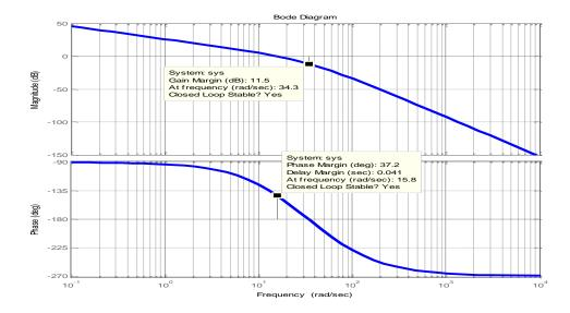
Phase margin(PM)= 37.22 deg. at 15.8 rad/sec; Gain margin(GM)= 11.5 dB at 34.3 rad/sec
